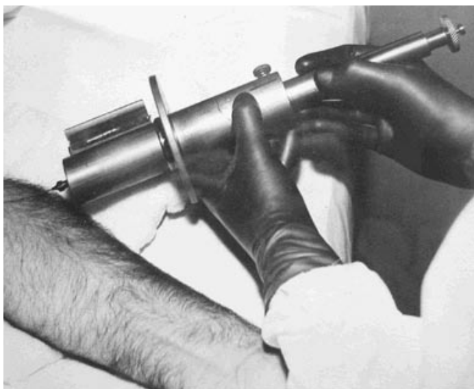
Syringe shield used for radioisotope injections during the late 1940s and early 1950s at the Oak Ridge Institute for Nuclear Studies.
